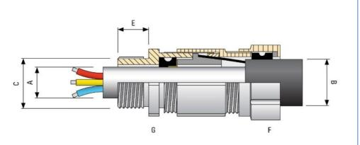
Designed to the B.S. 6121 standard, the IGE2W is a robust metallic range of cable glands for industrial applications which provides an outer and inner IP seal and armour clamping, grounding and earthing.
